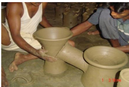
'Anagi' Stove, being made and installed with insulation
